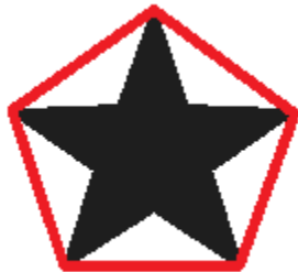
Figure 1: The red line would be the convex perimeter of a star shaped arm
